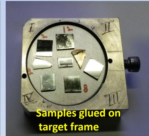
Samples glued on target frame
